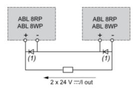
(1) Two Shottky diodes Imin = power supply In and Vmin = 50 V Parallel Connection
