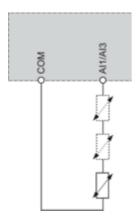
It is possible to connect either 1 or 3 sensors on terminals Al1 or Al3
