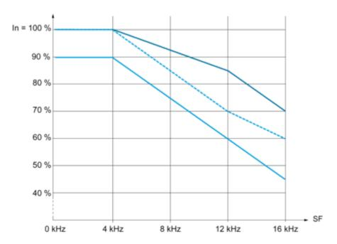
40 °C (104 °F) - Mounting type A, B and C 50 °C (122 °F) - Mounting type A, B and C 60 °C (140 °F) - Mounting type B and C
