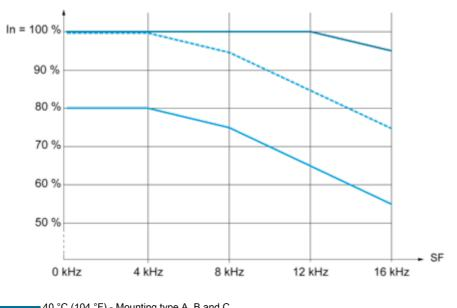
40 °C (104 °F) - Mounting type A, B and C 50 °C (122 °F) - Mounting type A, B and C 60 °C (140 °F) - Mounting type B and C In : Nominal Drive Current SF : Switching Frequency
