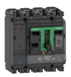
Circuit breaker ComPacT NSX100B, 25kA at 415VAC, TMD trip unit 80A, 50 degrees C, 4 poles 3D
