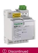
Residual current protection relay, VigiPacT RH10M, 50mA, 220/240VAC 50/60Hz, DIN rail mounting
