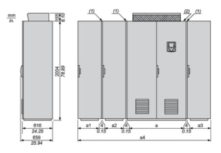
$(1) \qquad \mbox{Seal. For each floor-standing enclosure added, allow a 4 mm/0.15 in. space for the seal.}$
