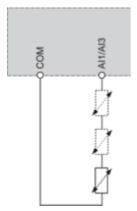
It is possible to connect either 1 or 3 sensors on terminals AI1 or AI3
