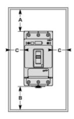
Toggle-type, rotary handle-type: identical clearance values.
