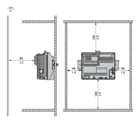
Keep adequate spacing for proper ventilation to maintain an ambient temperature between 0...50 °C (32...122 °F) for horizontal installation and 0...40 °C (32...104 °F) for vertical installation.
