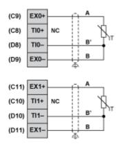
2 Wiring for Analog Inputs PT100
