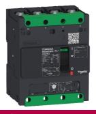
circuit breaker ComPact NSXm B (25 kA at 415 VAC), 4P 3d, 63 A rating TMD trip unit, compression lugs and busbar connectors
