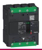
circuit breaker ComPact NSXm H (70 kA at 415 VAC), 4P 3d, 125 A rating TMD trip unit, EverLink connectors
