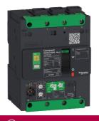
circuit breaker ComPact NSXm B (25 kA at 415 VAC), 3P 3d, 160 A rating Micrologic 4.1 trip unit, EverLink connectors
