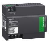
External power supply module, input voltage 200VAC to 240VAC 50/60Hz, output voltage 24VDC, output current 1A
