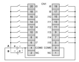
The COM0 terminals are connected internally
