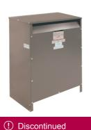
Transformer, dry type, 150kVA, 3 phase, 480V delta primary, 208Y/ 120V secondary, 24D, 80C rise, Cu
