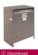
Transformer, dry type, 300kVA, 3 phase, 480V delta primary, 208Y/ 120V secondary, 30D, 80C rise, Cu
