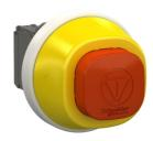
Antimicrobial Illuminated emergency stop, Harmony XB5, plastic, 22mm, trigger latching turn to release, white red LED, 24V AC DC, 1 NO + 1 NC
