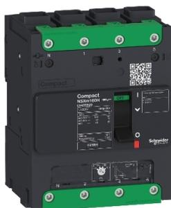
circuit breaker ComPact NSXm B (25 kA at 415 VAC), 4P 3d, 32 A rating TMD trip unit, EverLink connectors
