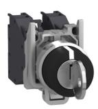
Key switch selector, metal, black, Ø22, key n°455, 3 positions, stay put, 2 NO
