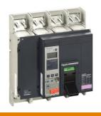
Circuit breaker, ComPact NS1600N, 50kA/415VAC, Micrologic 2.0E trip unit, 1600A, fixed, 4 poles 4d
