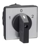
Cam changeover switch, Harmony K, front mounting, plastic, 2 poles, position 0, 30°, 32A, 64x64mm, marked 1/0/2
