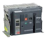
Circuit breaker frame, MasterPact NW12H1, 1250A, 65kA/440VAC 50/60Hz (Icu), 3 poles, drawout, without control unit
