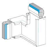
Edgewise and flat zed unit, Canalis KTA, aluminium, 3200A, 3L+N+PER (AI), made to measure, neutral N2, white RAL9001
