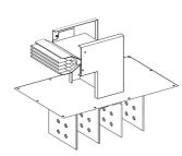
Flat elbow feed unit, Canalis KTA, aluminium, 3200A, 3L+PE, made to measure dimensions, neutral N4, white RAL9001
