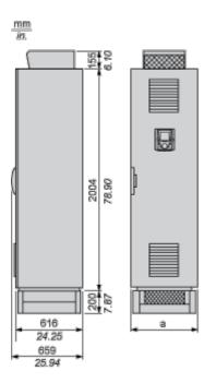
Standard Compact Floor-Standing Enclosure + Additional Floor-Standing Enclosures, According to the Configuration
