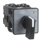
Cam changeover switch, Harmony K, Ø 22mm, plastic, 1 pole, 2 positions, 30°, 12A, 45x45mm, metallic legend, marked 1/2, 35mm black handle
