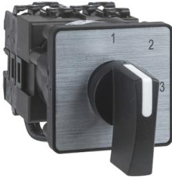
Cam stepping switch, Harmony K, multifixing, plastic, 3 poles, 2 steps, 45°, 12A, 45x45mm, metallic legend, marked 1/2, 35mm black handle
