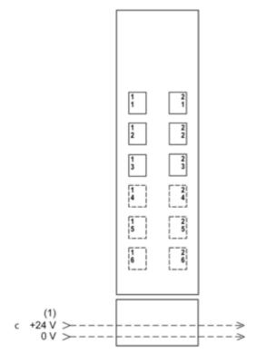
1 24 Vdc I/O power segment integrated into the bus bases
