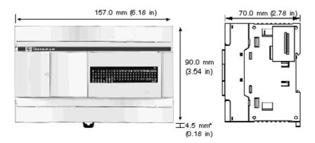
\* 8.5 mm (0.33 in) when the clamp is pulled out.
