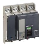
circuit breaker Compact NS800N, 50 kA at 415 VAC, Micrologic 2.0 trip unit, 800 A, fixed, 4 poles 4d
