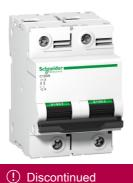
Miniature circuit breaker (MCB), Acti9 C120N, 2P, 63A, B curve, 10000A (IEC/EN 60898-1), 10kA (IEC/EN 60947-2)
