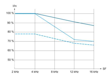
40 °C (104 °F) - Mounting type A, B and C 50 °C (122 °F) - Mounting type C 60 °C (140 °F) - Mounting type C
