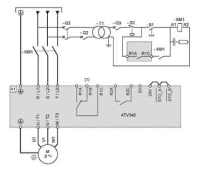
(1) Use relay output R1 set to operating state Fault to switch Off the product once an error is detected.
