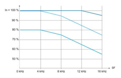
40 °C (104 °F) - Mounting type A, B and C 50 °C (122 °F) - Mounting type A, B and C 60 °C (140 °F) - Mounting type B and C In : Nominal Drive Current SF : Switching Frequency
