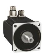
servo motor BMH, Lexium 32, 8.4Nm, 6000rpm, keyed shaft, without brake, IP54, 128bit encoder, straight
