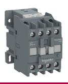
Contactor, Easy TeSys Control, LC1E, 3P(3NO),AC-3,<=440V,6A,380V AC coil,60Hz,1NC auxiliary contact
