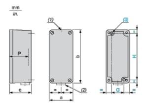
(1) 1 hole, without blanking plug, for cable gland with 14 mm/0.55 in. maximum clamping capacity
