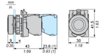
e: clamping thickness: 1 to 6 mm / 0.04 to 0.24 in. (1) Additional row of contacts or double contact
