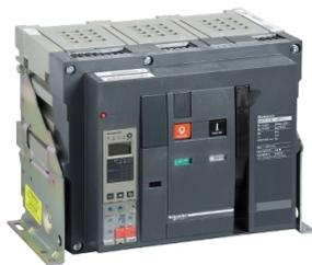
Circuit breaker frame, MasterPact NW32H2, 3200A, 100kA/440VAC 50/60Hz (Icu), 3 poles, drawout, without control unit
