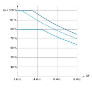
40 °C (104 °F) - Mounting type A, B and C 50 °C (122 °F) - Mounting type A and C 60 °C (140 °F) - Mounting type C In : Nominal Drive Current
