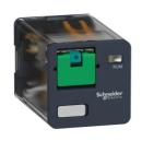
Harmony, Universal plug-in relay, 10 A, 2 CO, with lockable test button, flat (faston) terminals, 48 V DC
