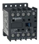
Contactor, TeSys K, 3P, AC-3/ AC-3e,<=440V 6A, aux. 1NC, 230...240V AC coil
