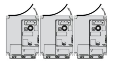
Mounting Type C: Individual, Ventilation Cover Removed
