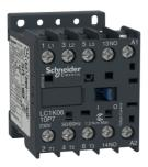
Contactor, TeSys K, 3P, AC-3/ AC-3e,<=440V 16A, aux. 1NO, 230...240V AC coil
