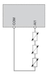
It is possible to connect either 1 or 3 sensors on terminals Al1.
