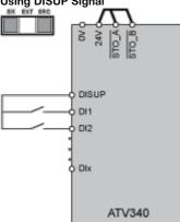
In SRC position DISUP outputs 24 V. In SK position DISUP is connected to 0 V.
