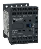
Control relay, TeSys K, 2NO+2NC, <= 690V, 230V AC coil, with integral suppression device, spring terminal
