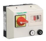
Enclosed DOL starter, TeSys LG, 2.5-4A, 220/230V AC coil, including 1 LC1K, GV2ME, rotary isolation switch, 2 pushbuttons
