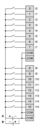
The 4 COM terminals are connected internally
