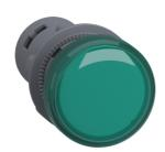
Monolithic pilot light, Easy Harmony XA2, plastic, green, 22mm, integral LED, screw clamp terminals, 220...230V AC, anti interference
